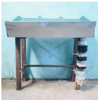
A. Rainwater Filter
